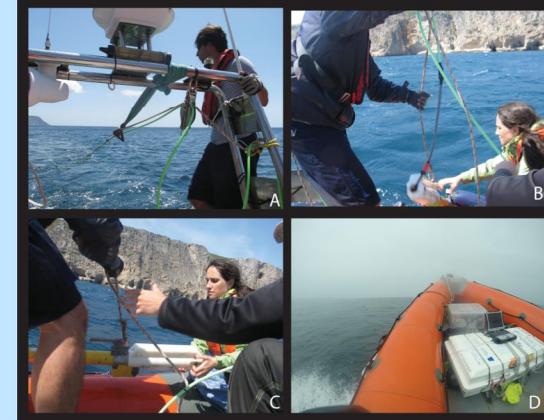
(A) Traction cable (white) winched at the boat stern, and both cables being towed. (B) Recovery of the fish to the boat, by pulling the traction cable. (C) Traction cable knotted to the magnetometer's hold. (D) The boat prow and the logging computer.
